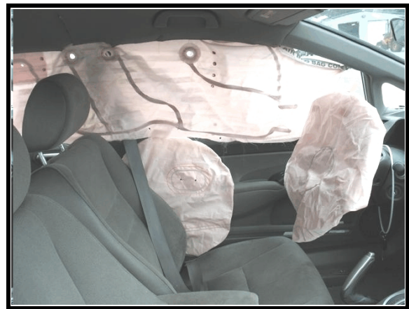
Figure 6. View showing deployed air bags
