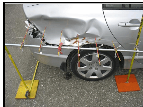
Figure 4. Right side damage
