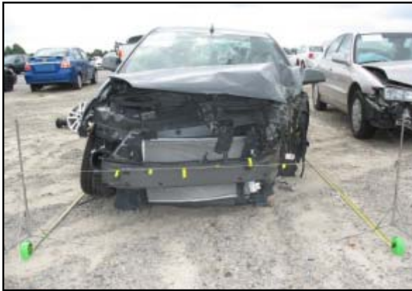
Figure 6. Residual frontal damage.
