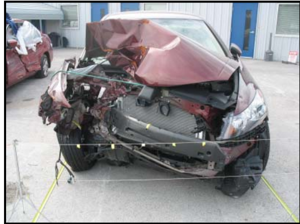
Figure 4: View of the Honda's frontal damage.
