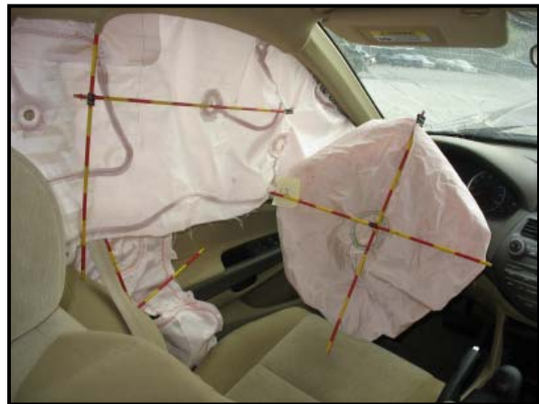
Figure 6: Deployed air bags in the driver's position.
