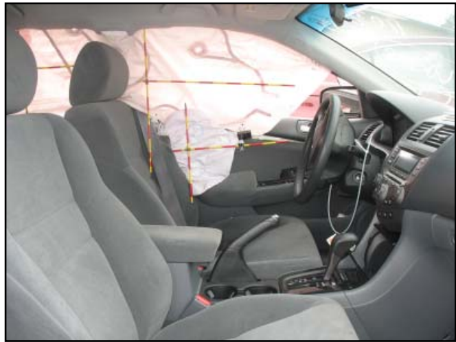
Figure 6: Right interior view of the deployed air bags at the driver's position.
