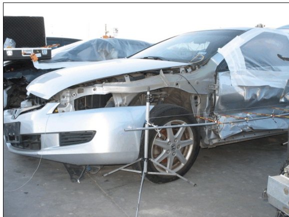
Figure 6: Honda's left side crush from impact by Chevrolet; C 6 was located just behind left front wheel assembly
