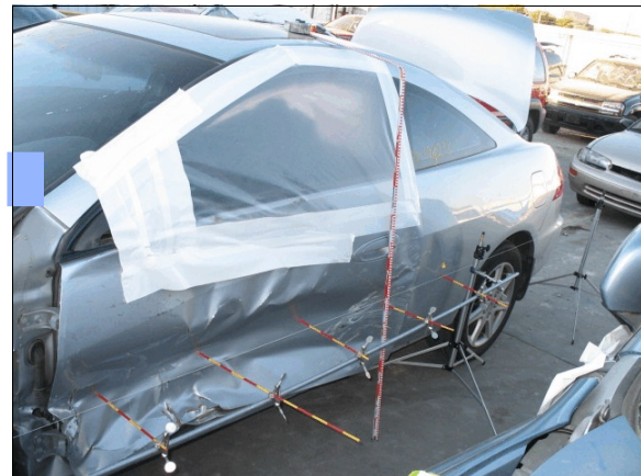
Figure 7: Elevated view from front of Honda's left side crush showing C 1 through C 5
