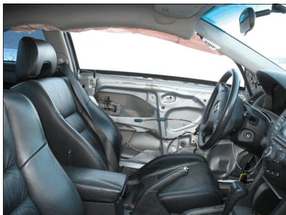
Figure 11: Honda's front seating area showing removed interior surface of driver's door and undeformed steering wheel rim
