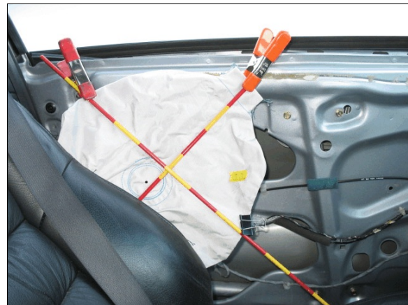
Figure 15: Inboard surface of Honda's deployed driver side air bag showing center circular stitching and deployment scuff toward front of bag
