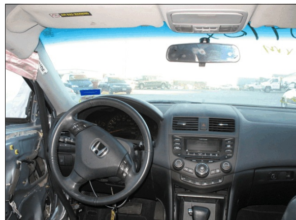
Figure 12: Honda's driver seating area showing no apparent occupant contact evidence or loading on steering wheel
