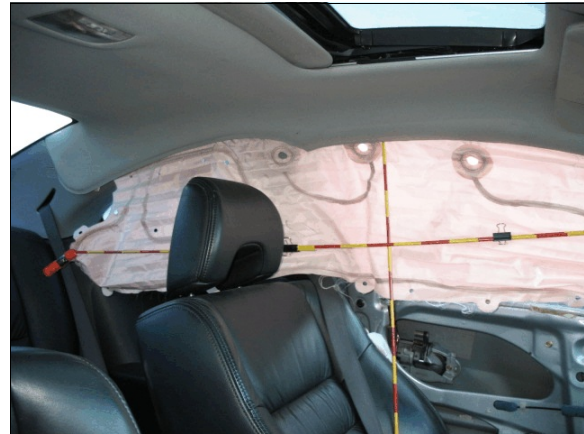
Figure 17: Rear and middle portions of Honda's deployed left IC air bag
