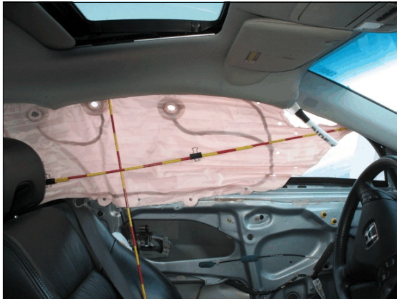
Figure 16: Front portion of Honda's deployed left IC air bag
