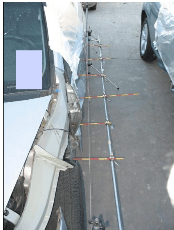
Figure 9: Elevated view of Honda's crush profile; C 6 was located just behind left front tire; maximum crush occurred at C 4
