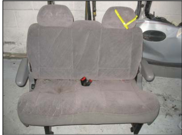
Figure 13: View of the contact to the left head restraint of the second row seat.
