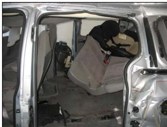
Figure 15: View of the second row seat and installed CRS.
