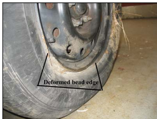
Figure 8: View of the deformed left rear wheel rim.
