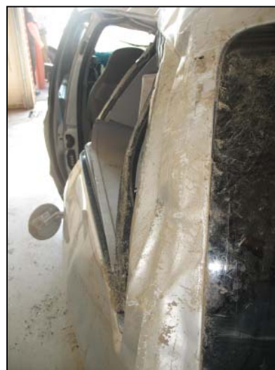
Figure 9: View the damage at the Ford's left D-pillar area.
