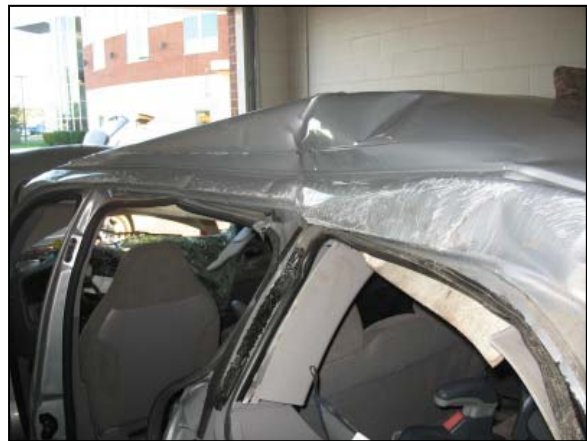
Figure 11: View of the maximum lateral deformation at the Ford's left roof side rail.
