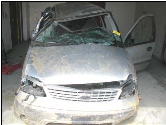
Figure 10: Front overall view of the Ford's rollover damage and maximum vertical damage at the right A-pillar.
