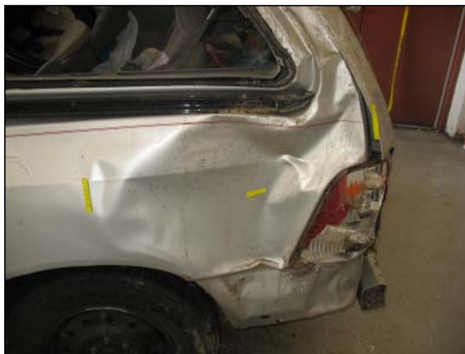
Figure 12: View of the isolated damage to the Ford's left quarter panel.
