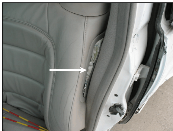
Figure 9: Arrow shows the location of the left front seat back-mounted side impact air bag
