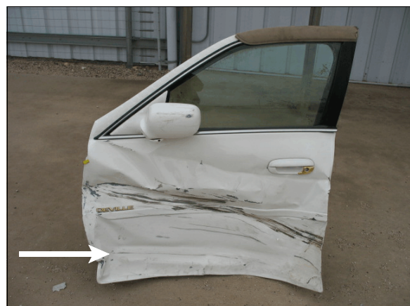
Figure 4: Direct damage to the 2001 Cadillac's left front door from impact with the 2005 Cadillac; arrow shows level of bumper contact
