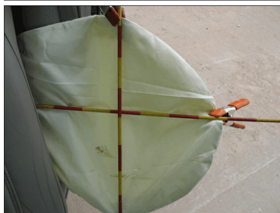
Figure 10: The deployed left front seat back-mounted side impact air bag
