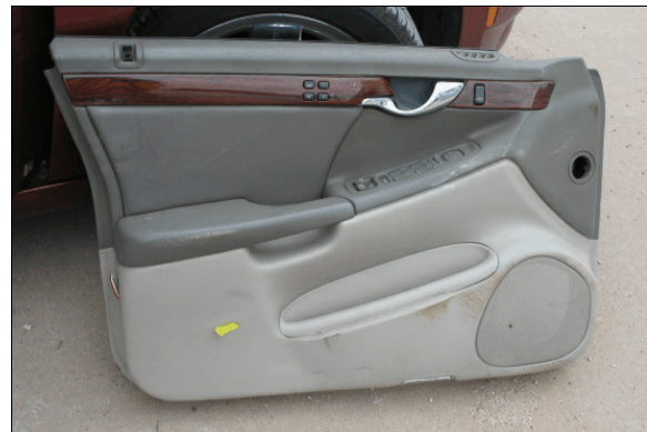
Figure 8: Left front door panel; yellow tape shows dent from contact with seat control panel on driver’s seat
