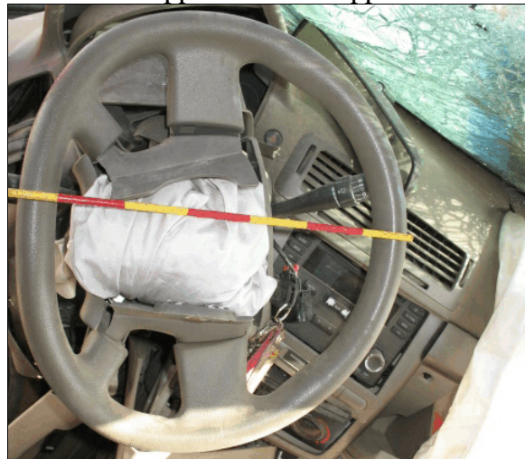
Figure 13: The steering wheel and air bag module cover flaps; steering wheel rotated 90 degrees clockwise
