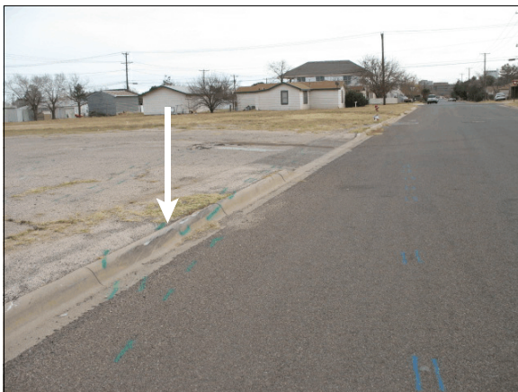
Figure 10: Arrow shows tire mark and scrapes on the curb from impact by the Cobalt's left rear wheel
