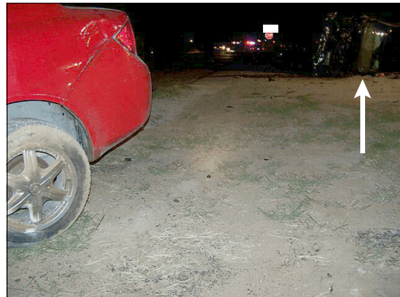
Figure 9: Police photo of Cobalt's left rear wheel showing abrasions to tire sidewall and rim scratches from curb impact; arrow shows final rest position of the Silverado
