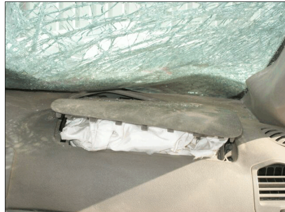
Figure 15: The front right passenger's frontal air bag cover flap and air bag module)
