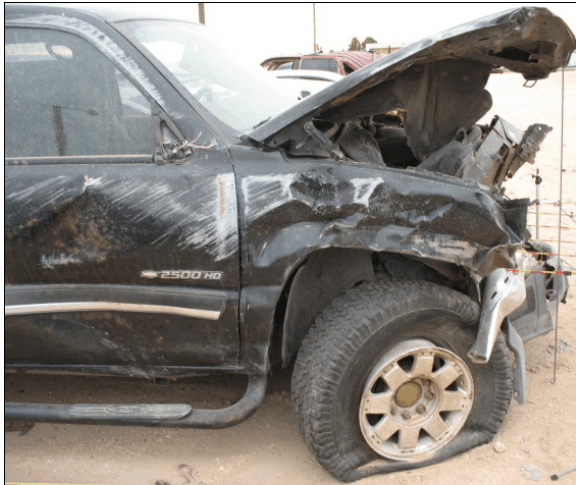
Figure 8: Damage to Silverado's door and fender from impact with the Cobalt's left quarter panel and left rear door; tire deformed from curb impact
