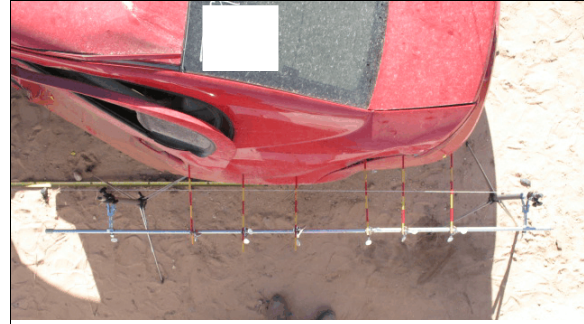
Figure 7: Top view of damage on the rear portion of the Cobalt's left rear door and the quarter panel from impact with the Silverado's right front door and fender
