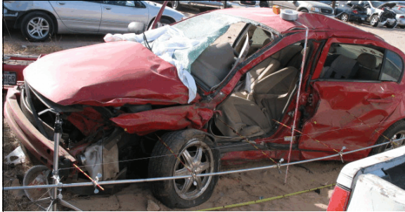
Figure 6: Damage to the left side plane of the Cobalt from impact with the front of the Silverado
