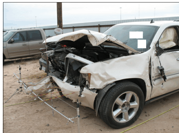
Figure 4: Damage to the front plane of the Chevrolet due to the impact with the right side plane of the Hyundai
