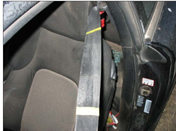
Figure 13: Load abrasion on the driver’s seat belt
