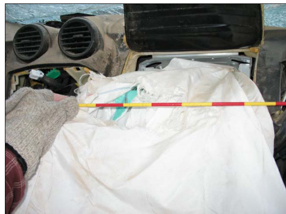
Figure 10: Tear in top of front right passenger's frontal air bag
