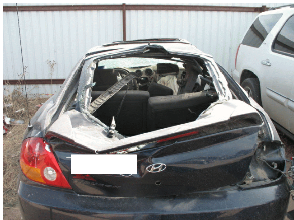
Figure 5: Damage to the top plane on the back of the Hyundai due to impact from the Chevrolet as it rolled over
