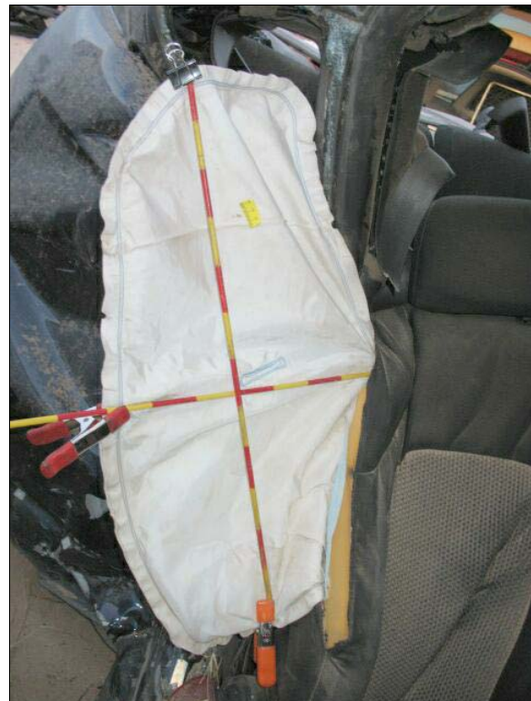
Figure 12: The deployed front right seat back-mounted side impact air bag
