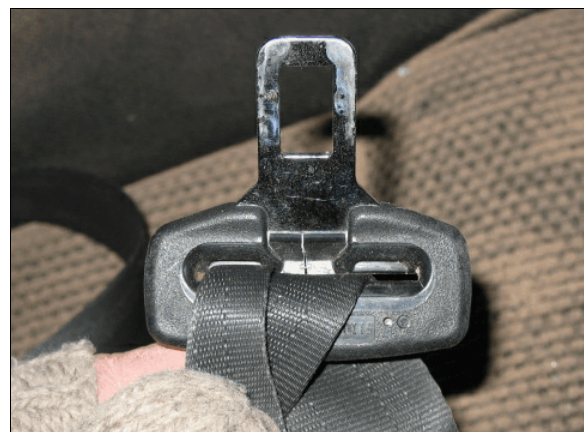
Figure 14: The front right passenger’s seat belt webbing was folded over on itself and jammed in the latch plate belt guide
