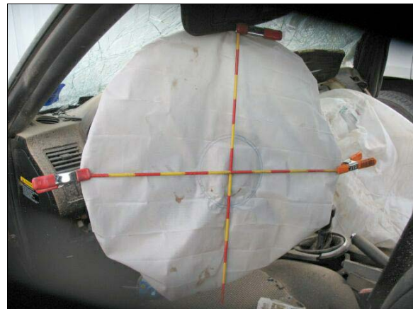
Figure 9: The driver's deployed frontal air bag
