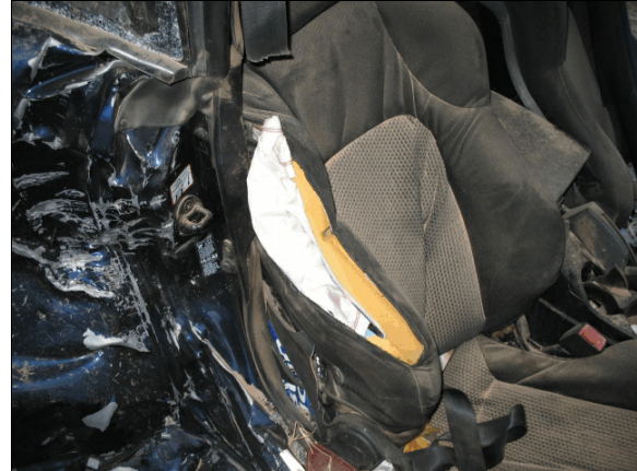
Figure 11: Location of the Hyundai's front right passenger's seat back-mounted side impact air bag
