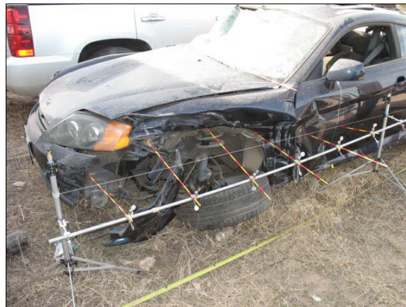
Figure 6: Hyundai's damage from impact with parked Ford Taurus
