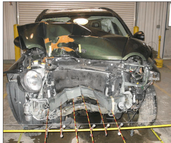
Figure 4: Damage to the front of the Jeep from impact with the tree
