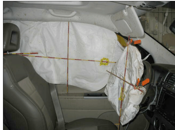
Figure 10: Driver's portion of the left IC air bag; yellow tape shows small transfer of makeup
