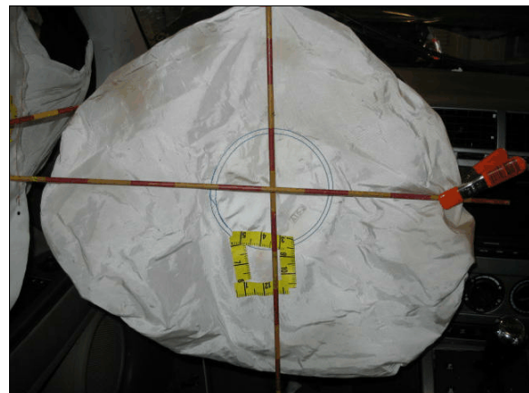
Figure 9: The driver's frontal air bag; yellow tape shows makeup transfer on the air bag
