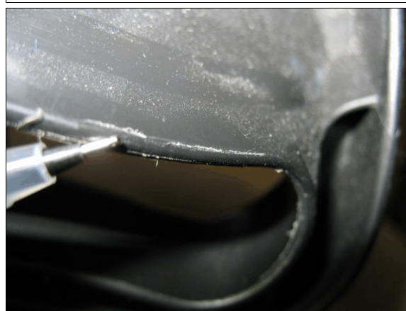
Figure 15: Safety belt abrasion on top back of BBS's right shoulder belt guide
