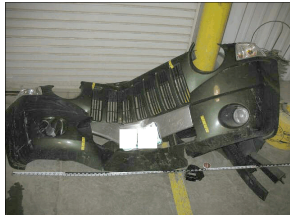
Figure 6: Yellow tape shows ends of direct contact damage on the front bumper fascia
