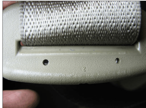
Figure 13: Load abrasion on second row right passenger's latch plate belt guide
