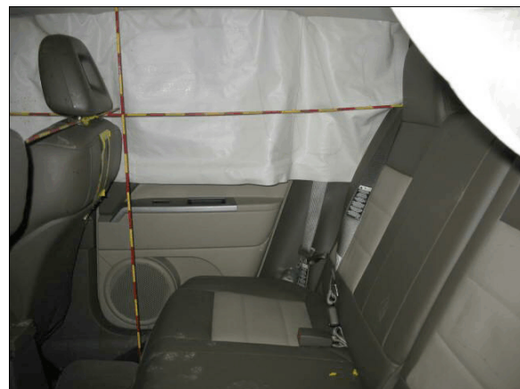
Figure 12: Second row right portion of right IC air bag
