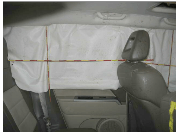
Figure 11: Second row left portion of left IC air bag
