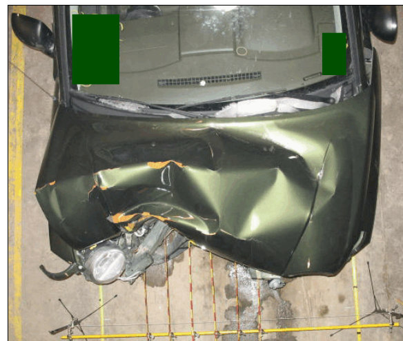
Figure 7: Crush to the front of the Jeep from the tree impact
