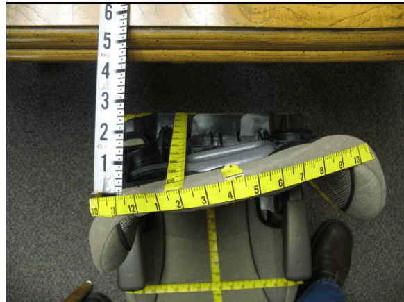
Figure 17: Top view of deformation to the BBS's head restraint
