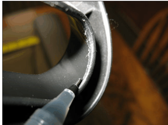
Figure 16: Safety belt abrasion on back inside surface of BBS's right shoulder belt guide
