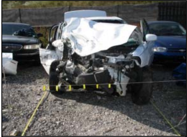
Figure 7. Overall view of the Chevrolet's frontal crush profile.
