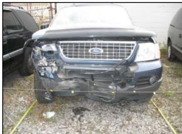
Figure 12. Frontal damage from the wall impact.
