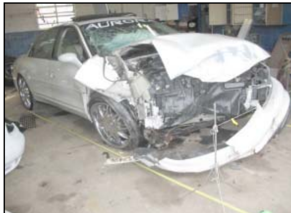
Figure 10. Resultant damage to the front of the Oldsmobile.
