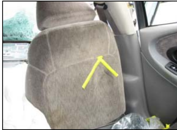
Figure 9. Occupant contact to the rear of right front seat back.
