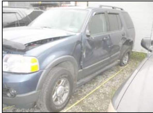
Figure 11. Overall view of the left side damage.
