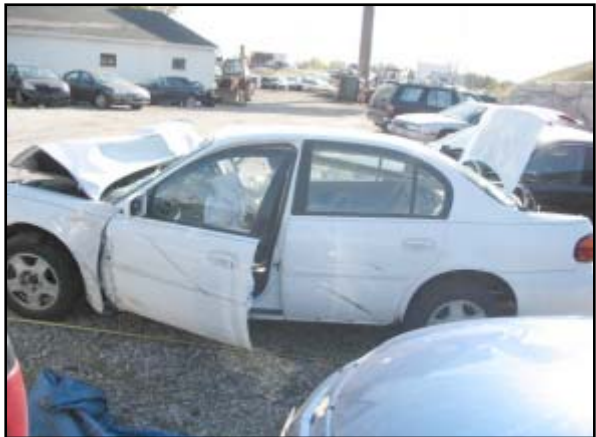
Figure 8. Left side damage to the Chevrolet from the impact with the Ford.
