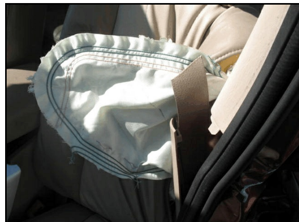
Figure 7: Driver's seat-mounted side impact air bag, showing the outboard surface of the air bag and the stub of the driver's safety belt, which was cut by emergency response personnel
