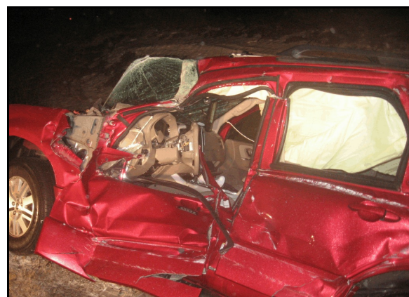
Figure 4: On-scene view of Mercury's left side damage, after extrication of the occupants
