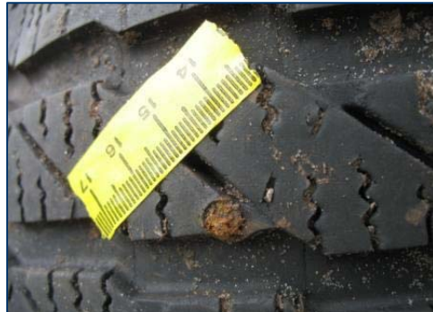
Figure 14. Steel object in the tread of the left rear tire.
