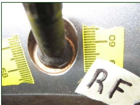
Figure 19. Crack/gouge to the base of the right front valve stem.
