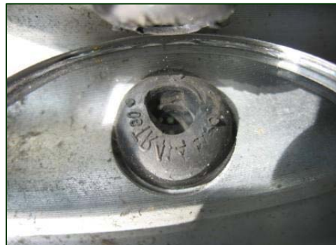
Figure 16. Identification numbers on the inside aspect of the left rear valve stem.
