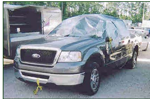
Figure 8. Left side rollover damage prior to the noted repairs (Image provided by the driver's attorney).
