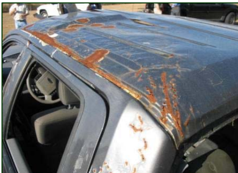
Figure 4. Partially repaired damage of the left roof side rail and C-pillar area.
