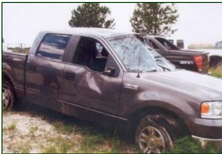
Figure 7. Right side rollover damage to the F150 (Image provided by the driver's attorney).
