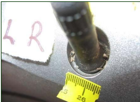
Figure 15. Lateral cracking of the left rear valve stem.
