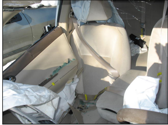
Figure 8: Contact point evidence on the Chevrolet's right/front door panel
