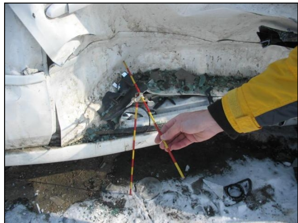
Figure 5: The right side crush profile of the Chevrolet.
