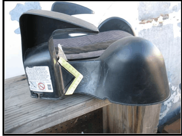
Figure 14. Right side BSS damage
