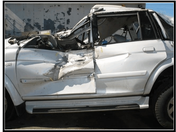
Figure 6. Left side damage from guardrail
