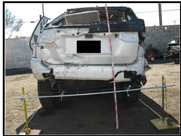
Figure 5. Rear end damage
