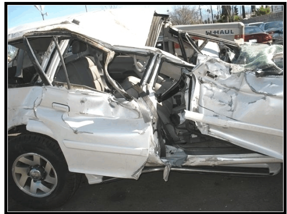
Figure 7. Right side damage from pole
