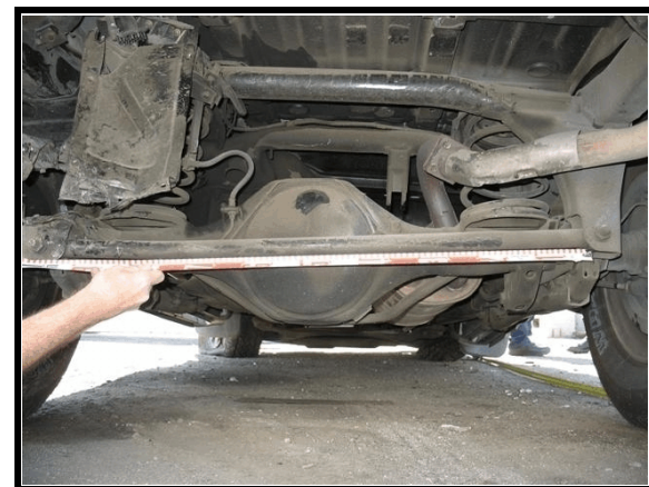
Figure 4. Rear axle stabilizer contact
