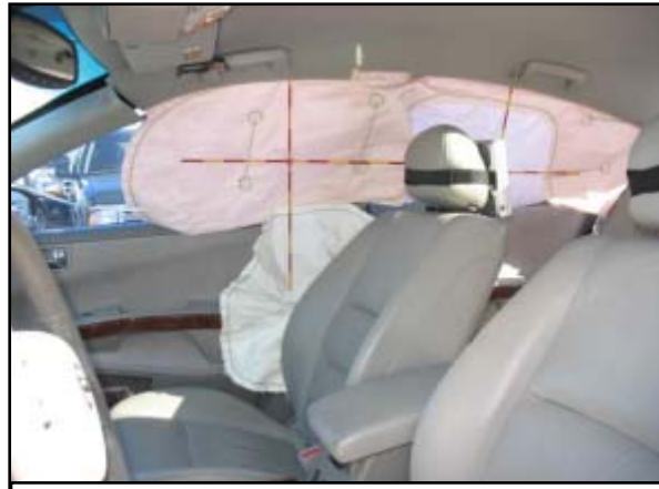
Figure 11. Deployed right side impact air bag system.
