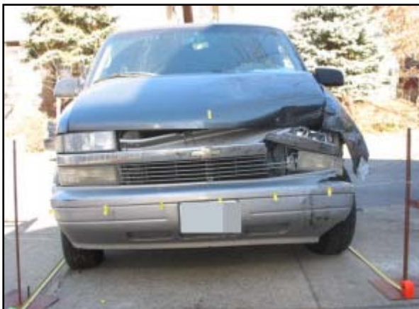
Figure 8. Residual frontal damage to the Chevrolet.
