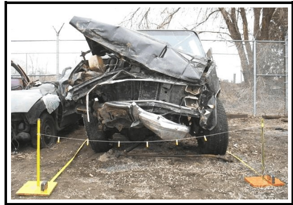
Figure 7. Front end crush profile measurement, 1985 GMC K3500
