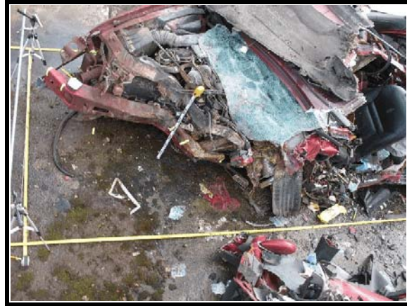
Figure 15. Overview of frontal damage
