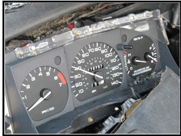
Figure 6. Lincoln speedometer needle position
