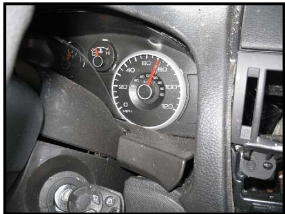
Figure 5. Ford speedometer needle position
