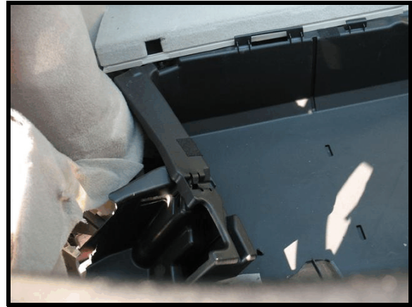
Figure 4. Cargo area intrusion
