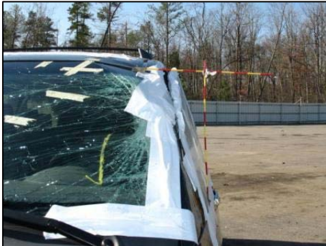
Figure 4. Lateral displacement of the left upper A-pillar with vertical displacement of the windshield header.
