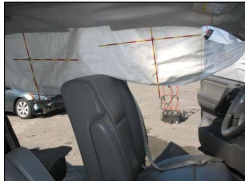
Figure 8. Deployed IC air bag in the driver's position of the Nissan.
