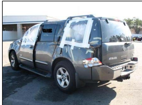
Figure 5. Lateral displacement of the left upper C-pillar and adjacent side rail.
