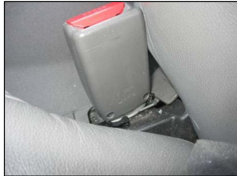
Figure 6. Actuation of the front left buckle pretensioner of the Nissan.
