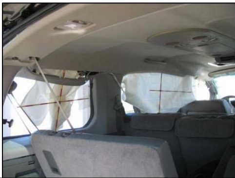
Figure 7. Overall view of the deployed left IC air bags in the Nissan.
