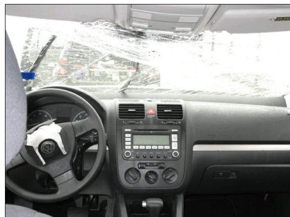
Figure 10: Intrusion of the windshield header and roof
