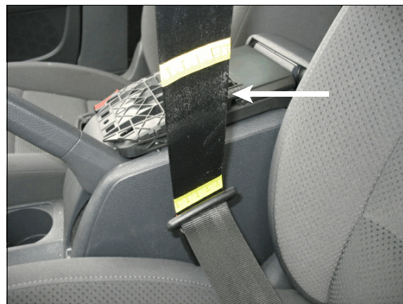
Figure 13: Load mark on driver’s seat belt
