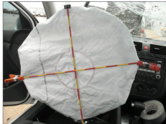
Figure 12: The driver’s deployed frontal air bag
