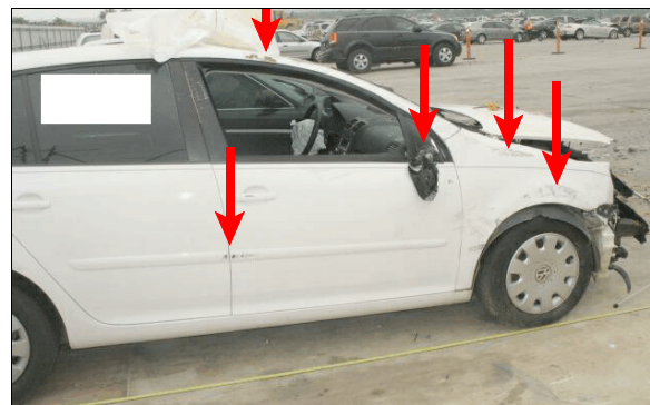
Figure 4: Arrows show damage to the right side plane due to the rollover.
