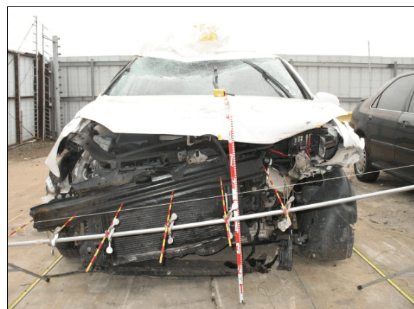
Figure 3: Damage to the front plane of the Volkswagen due to impact with the concrete Jersey barrier and on the roof due to the rollover
