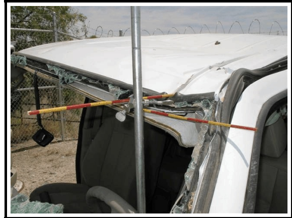
Figure 3. Maximum vertical crush measurement, left windshield header
