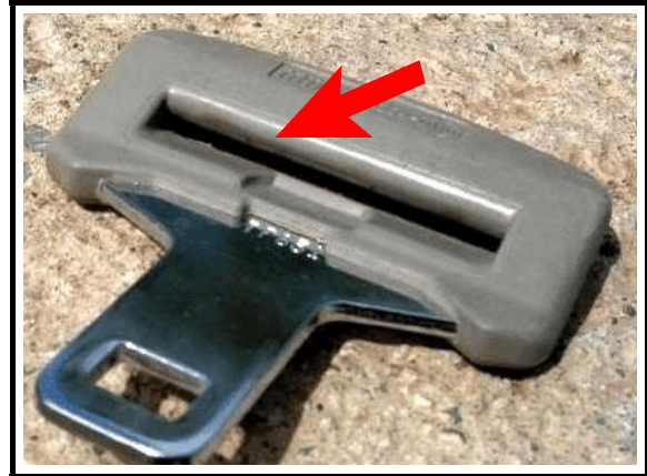
Figure 4. The driver's safety belt latch plate showing loading evidence
