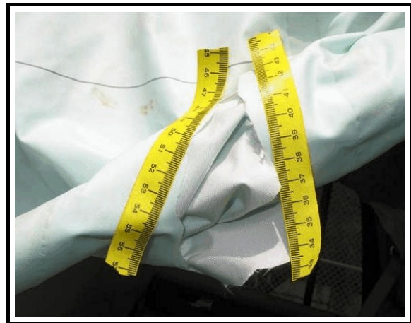
Figure 6. Damage to left IC air bag
