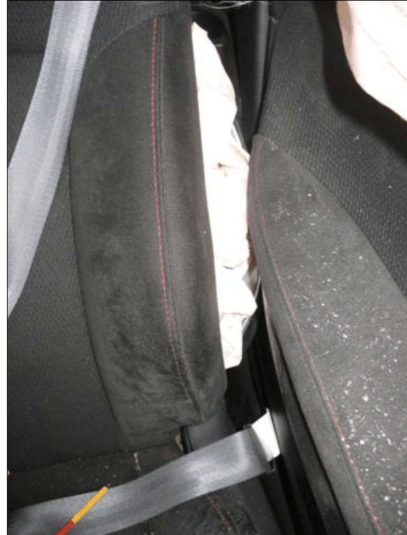
Figure 8: The location of the front left seat-mounted side impact air bag
