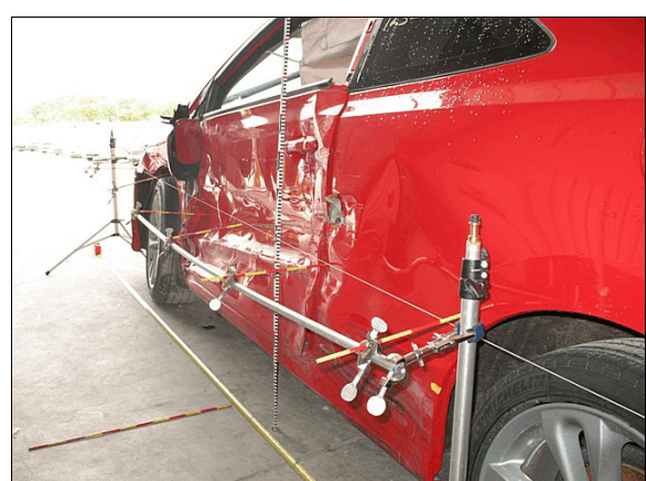
Figure 5: Damage on the left side lane of the Honda from the impact with the Toyota
