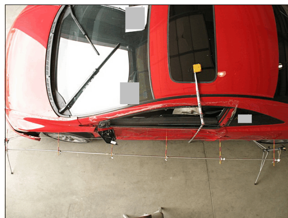
Figure 6: Top view of the crush on the left side plane of the Honda
