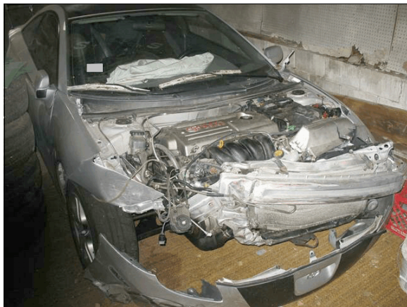
Figure 4: Damage on the front plane of the Toyota from the impact with the left side plane of the Honda
