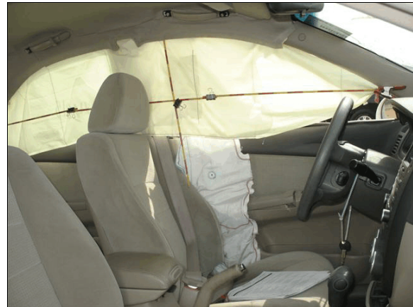
Figure 8: The left side impact IC air bag and left front seat-mounted side impact air bag
