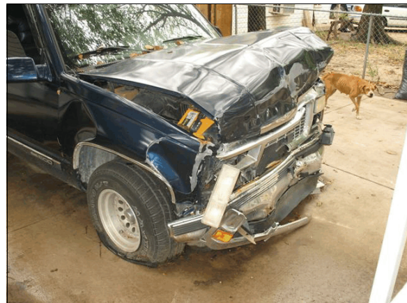
Figure 4: Front damage on the GMC from the impact with the left side plane of the Kia
