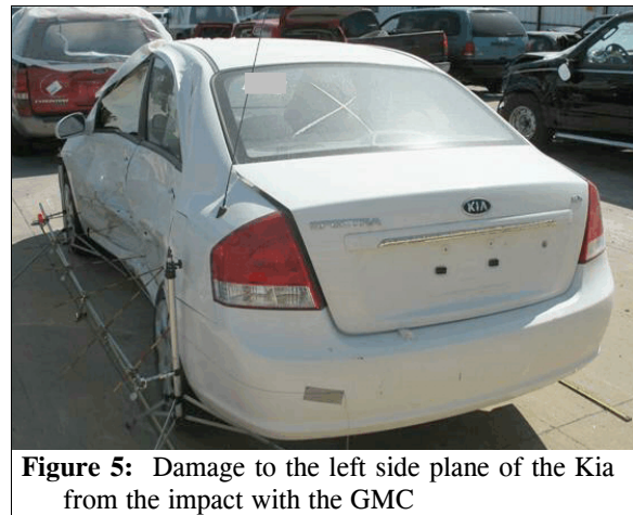
Figure 5: Damage to the left side plane of the Kia from the impact with the GMC
