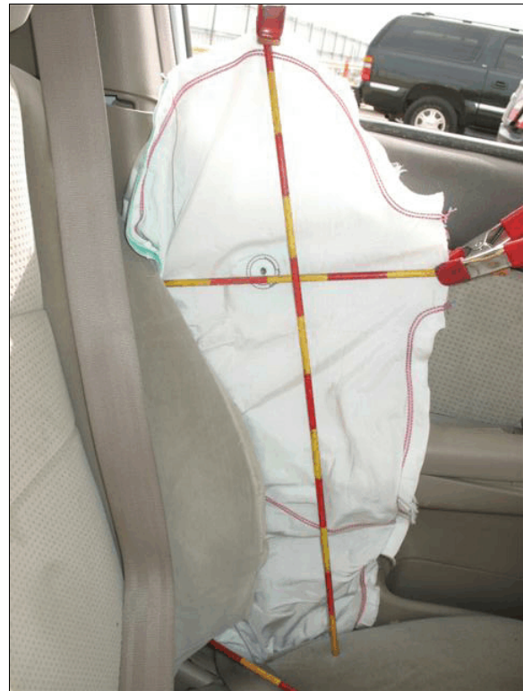
Figure 10: The left front seat-mounted side impact air bag
