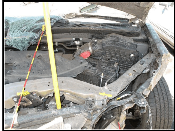
Figure 8. Left upper bulkhead frame
