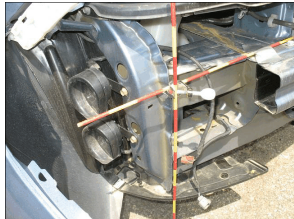
Figure 9: View of undamaged ACE components on front right
