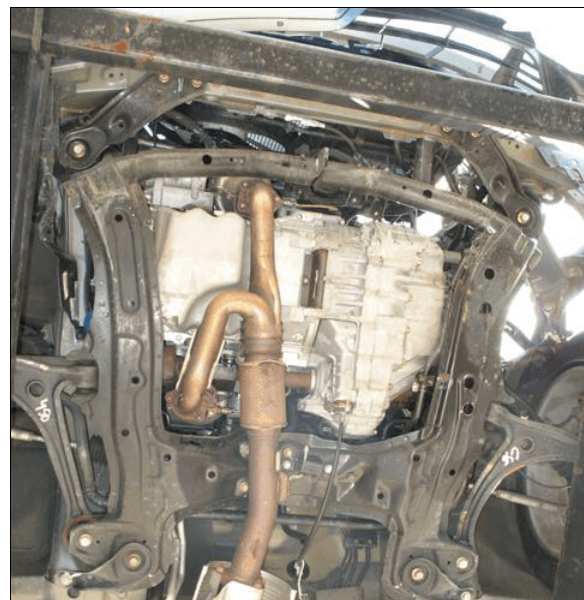
Figure 11: Undercarriage view of the left front wheel, suspensions components, engine, and stub frame
