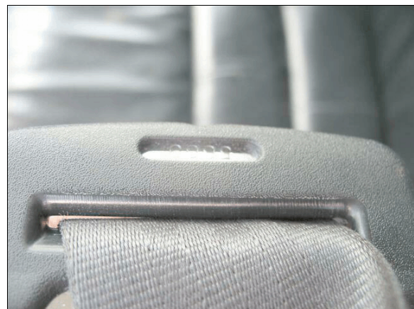
Figure 16: Light load abrasions on the driver's latch plate belt guide
