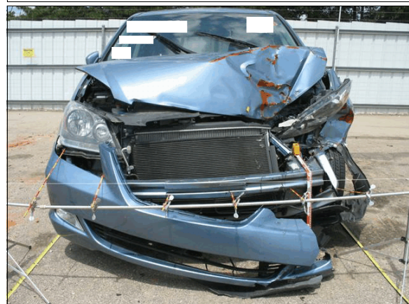
Figure 4: Front plane damage on the Honda from the impact with the back plane of the Ford
