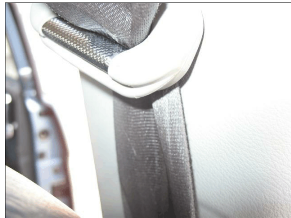
Figure 15: The driver's safety belt webbing was entrapped in the forward corner of the D-ring
