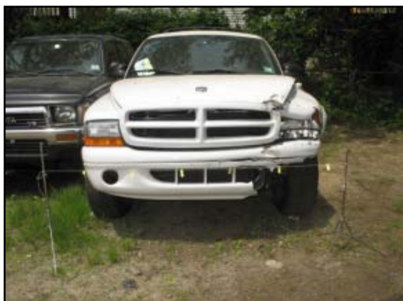
Figure 7. Frontal damage to the 2000 Dodge Durango.
