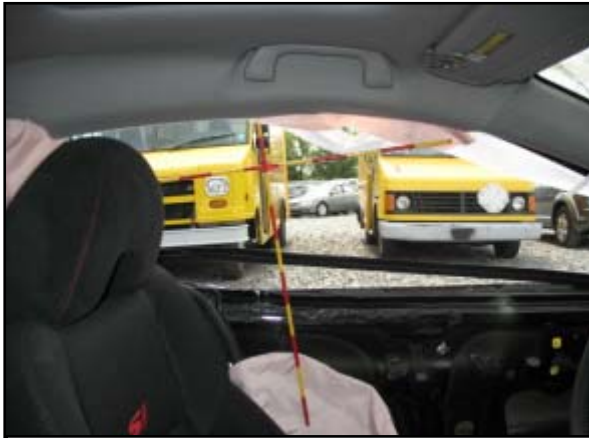
Figure 8. Curtain air bag cut from the left front position.
