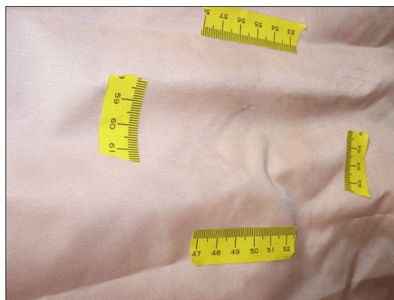
Figure 9: Tape outlines area of make-up transfer on the driver's frontal air bag
