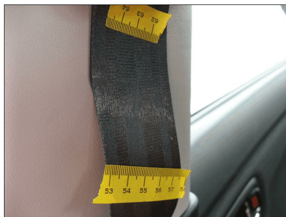
Figure 12: Friction abrasion on the belt webbing of the Mazda’s front passenger
