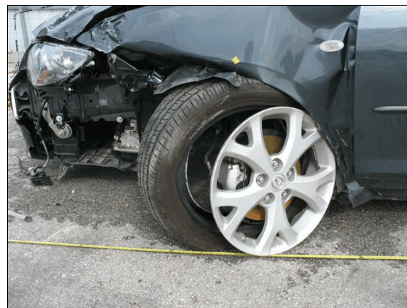
Figure 7: The impact displaced the Mazda's left front wheel rearward 20 cm (7.8 in)
