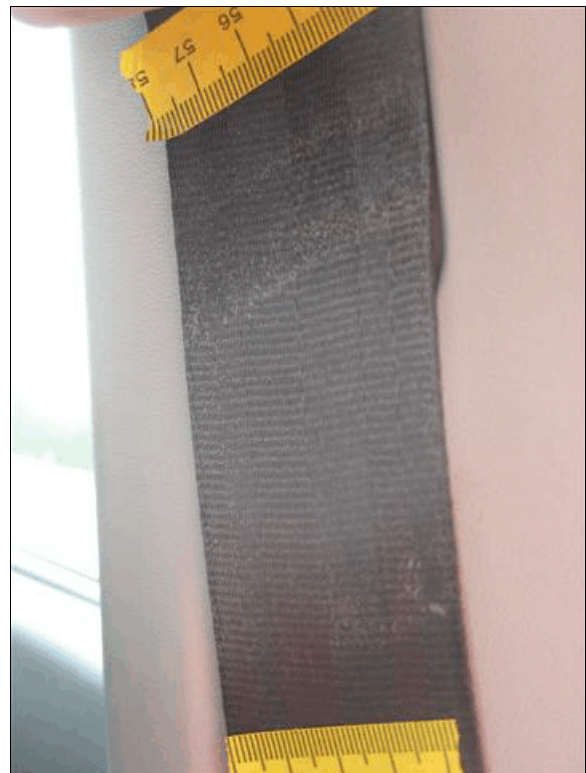
Figure 11: Abrasion on the belt webbing of the Mazda's driver
