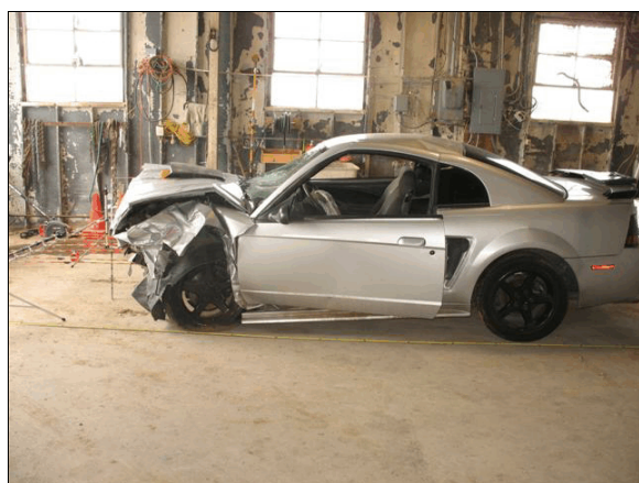
Figure 15: Left side view of the front plane damage on the Ford
