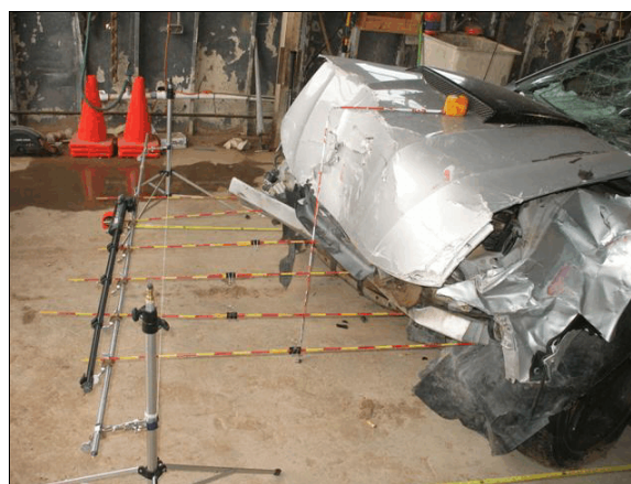
Figure 16: Left side view of the front plane crush on the Ford
