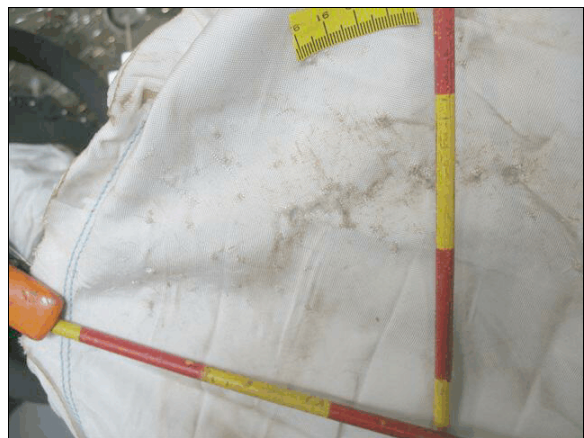
Figure 13: Abrasions and small holes on the forward upper quadrant of the left seat-mounted side impact air bag due to contact by glass fragments from the disintegrated left front window glazing
