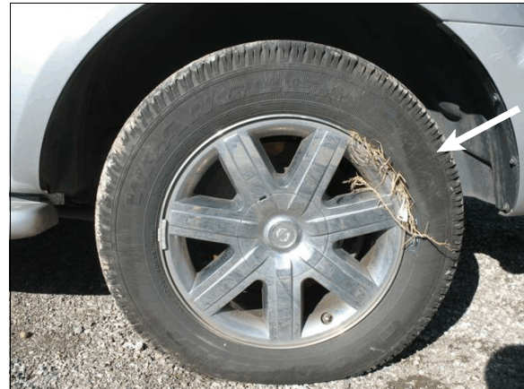
Figure 7: Abrasions on sidewall of the Chrysler’s left rear tire and grass embedded in the bead
