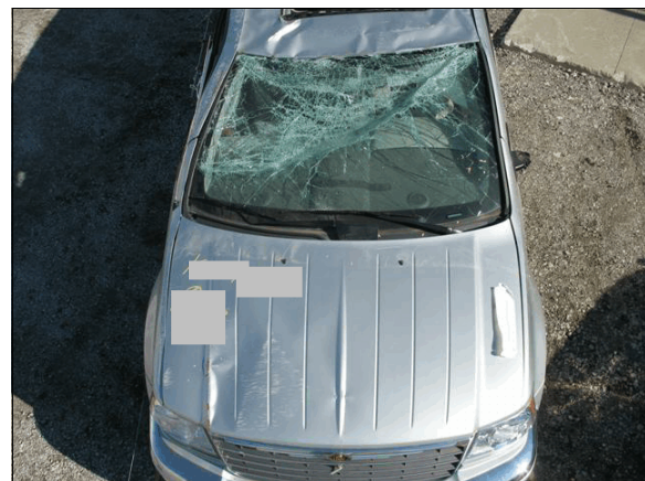
Figure 8: Direct damage to the hood, windshield, and front portion of the roof from the rollover
