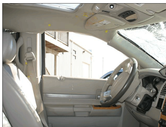
Figure 13: Yellow tape shows areas of occupant contact on the sunvisor, roof, and left roof side rail
