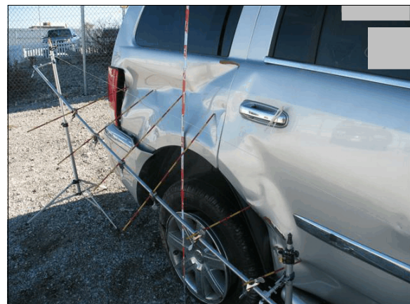
Figure 4: Damage to the right quarter panel of the Chrysler from the impact by the front plane of the Dodge
