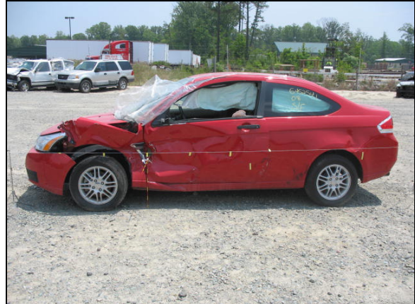
Figure 3: View of the crush profile on the left side of the Ford (Event 1).
