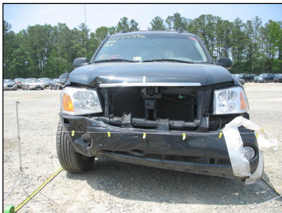
Figure 5: View of the crush profile on the front plane of the GMC (Event 1)
