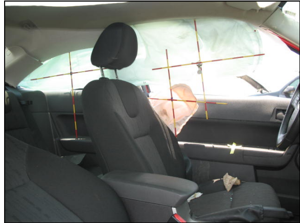
Figure 4: View of the left side (IC) air bag and the driver seatback mounted air bag in the Ford.
