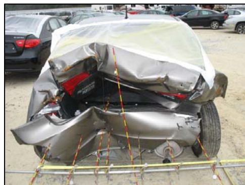
Figure 3: Damage to the rear of the Honda.
