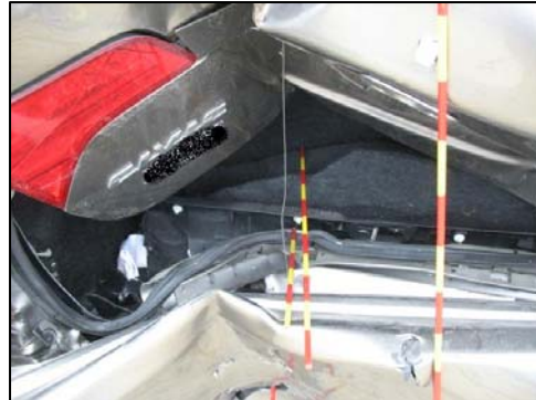
Figure 4: Distance remaining between maximum crush and the hybrid battery.
