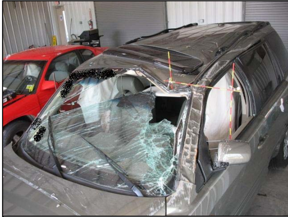
Figure 6: Honda rollover damage from above, left front.
