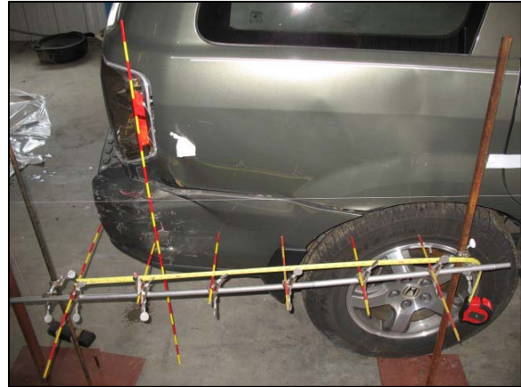
Figure 5: Secondary (Event 2) damage to the right rear of the Honda.
