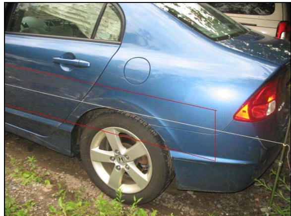
Figure 4: Depicts the side-swipe type damage from event 2
