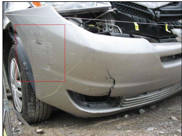
Figure 7: Right oblique view depicting the side-swipe damage from Event 2.
