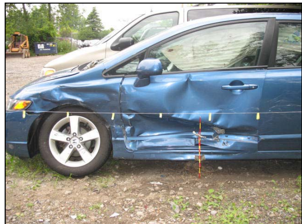
Figure 3: Close-up view of the Honda's impact damage.
