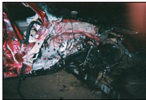
Figure 3. Right side view of the initial impact damage to the Ford.
