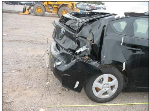
Figure 4: Right view at the back plane depicting the extent of crush.
