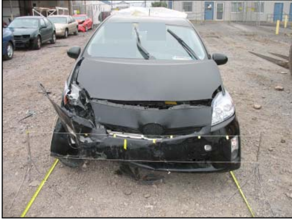
Figure 5: View of the frontal damage to the Toyota.
