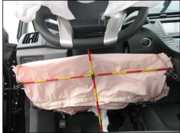
Figure 10: Deployed driver knee air bag.
