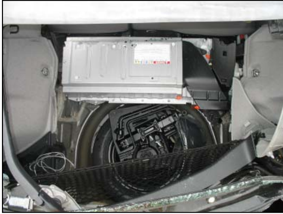
Figure 7: Overhead view through the disintegrated backlight of the cargo area and hybrid battery.
