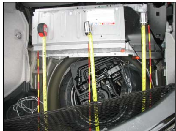
Figure 9: View depicting the relationship of the hybrid battery to the rear deformation of the
