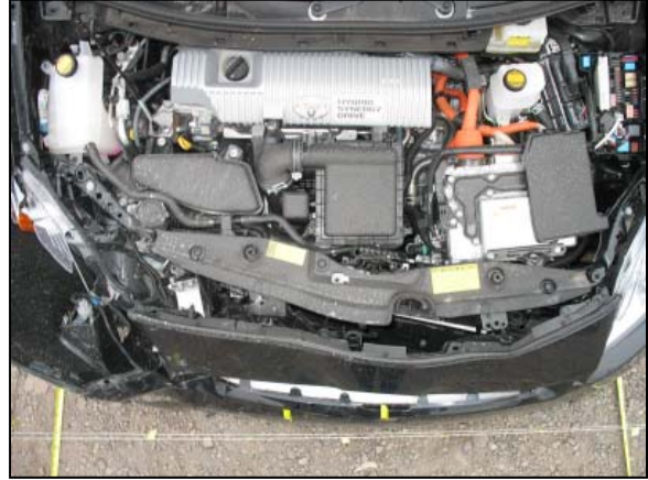
Figure 6: Overhead view of the frontal deformation.
