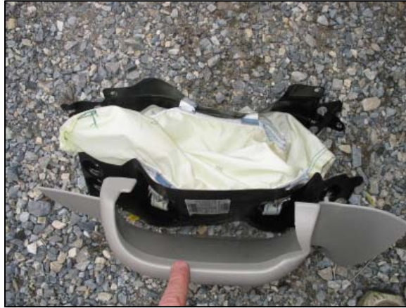
Figure 11: Overhead view of the knee air bag assembly removed from the vehicle.
