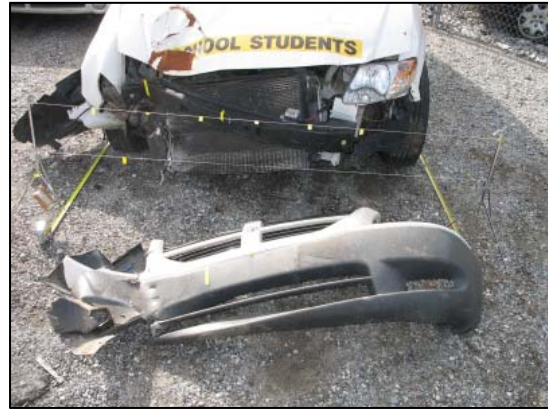
Figure 4: Front view of the damage to the Dodge Caravan resultant to the utility pole
