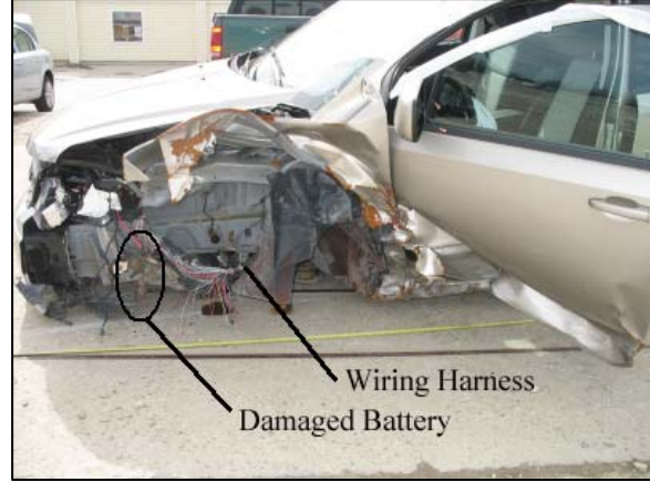
Figure 4: Left side view of the damage at the fender. Note the damaged battery and exposed/damaged wiring harness.
