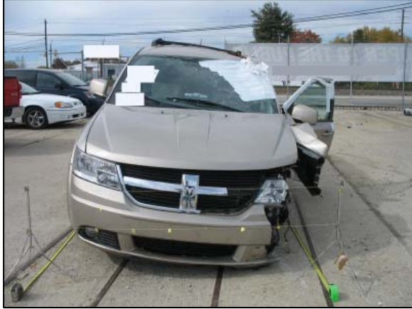
Figure 3: View of the frontal impact damage.
