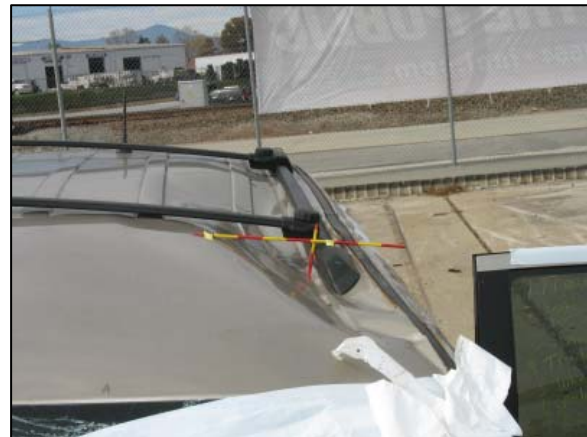
Figure 5: View of the deformed roof and the maximum vertical deformation adjacent to the B-pillar.
