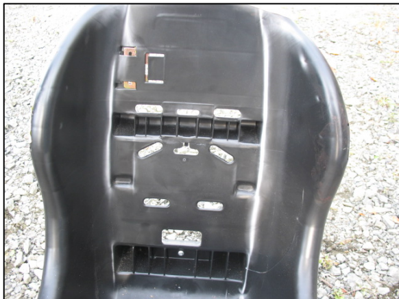
Figure 9: Loading stress marks distributed throughout the plastic shell of the CRS.
