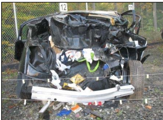
Figure 4: Rear view of the impact damage to the Saturn.
