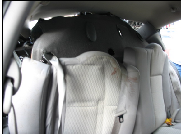
Figure 7: Depicts longitudinal intrusion of the second row seatback and rear shelf
