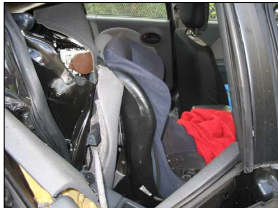
Figure 10: Post-crash position of the CRS.
