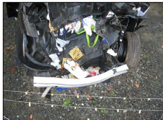
Figure 5: Overhead view of the Saturn's crush at the bumper level and the above bumper level.
