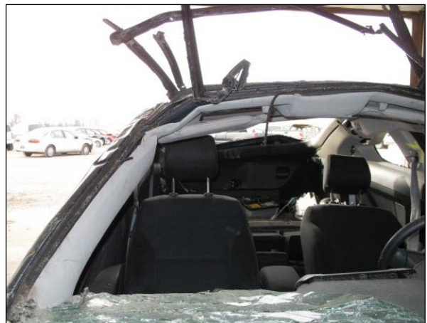
Figure 7: Maximum lateral crush to the right A-pillar of the Scion.
