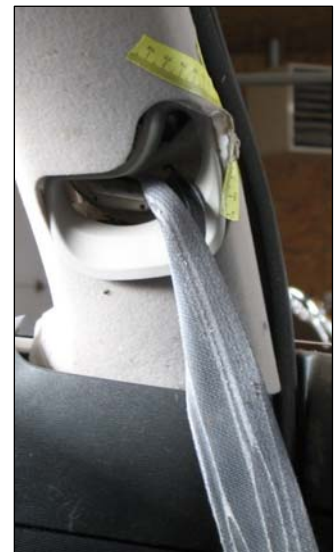
Figure 8: Upper safety belt webbing loading striations and B-pillar abrasions.
