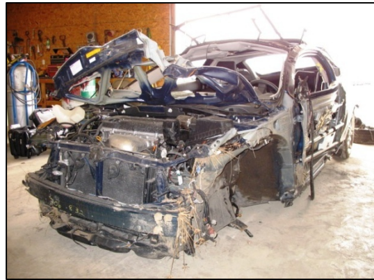
Figure 1: Left front oblique view of the rollover damage to the 2005 Scion tC.
