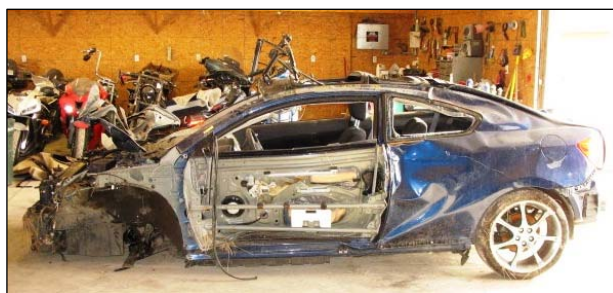
Figure 5: Left side view of damaged Scion.
