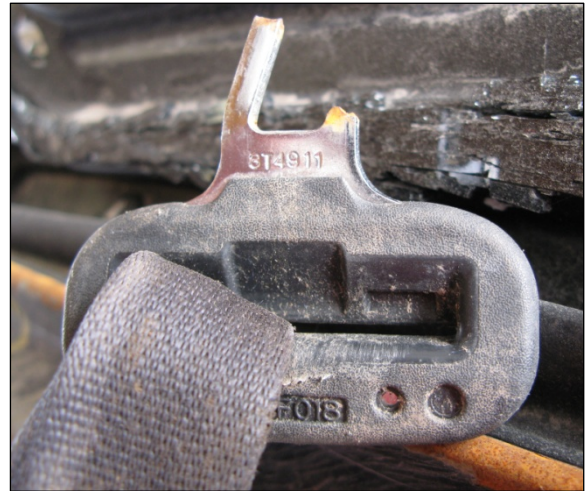
Figure 9: Latch plate loading evidence and fractured lock clasp.
