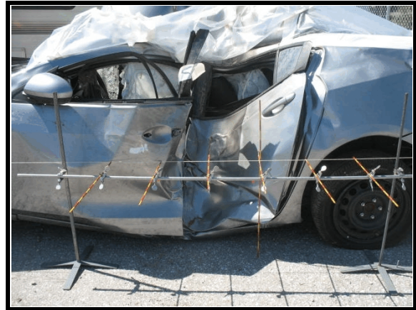
Figure 3. Left side pole damage
