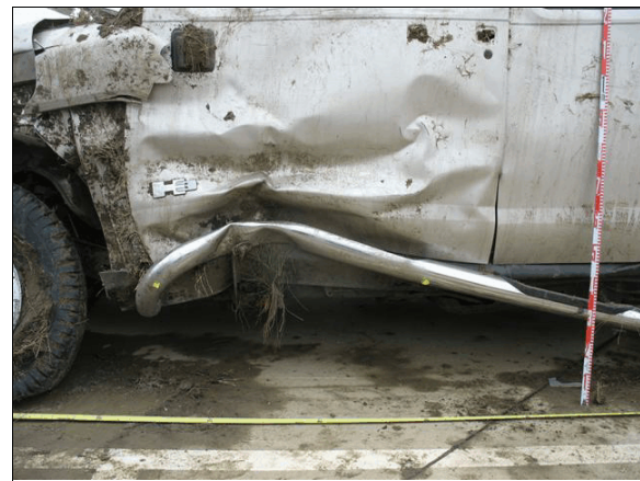
Figure 11: Damage on the left sill and undercarriage
