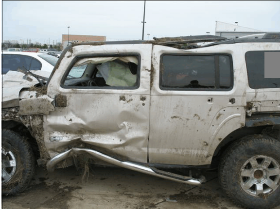
Figure 7: Damage on sill and undercarriage
