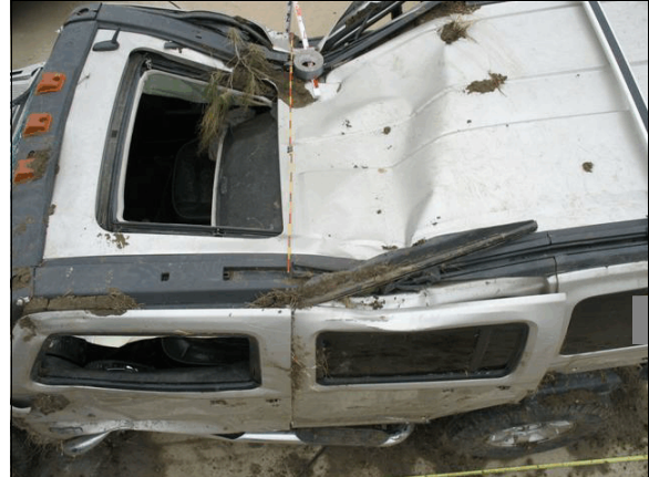
Figure 8: Damage to the top plane from impact with a pine tree during the rollover
