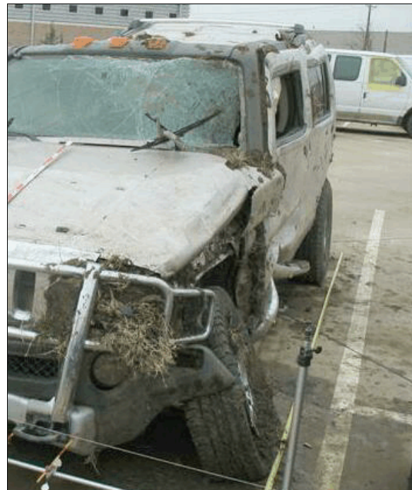
Figure 5: Mud deposits and damage on the front and left side plane from the rollover
