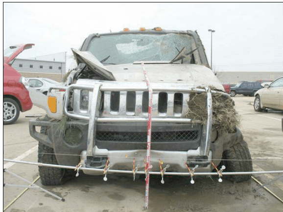
Figure 3: Damage on the front plane of the Hummer from the guardrail impact and rollover
