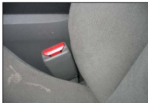
Figure 8: View of the actuated driver's buckle pretensioner.
