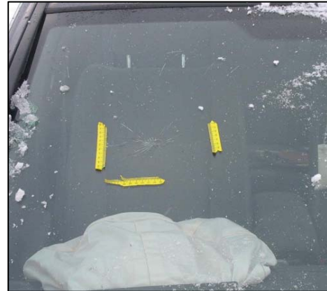
Figure 7: Fracture/cracks of the right aspect of the windshield.
