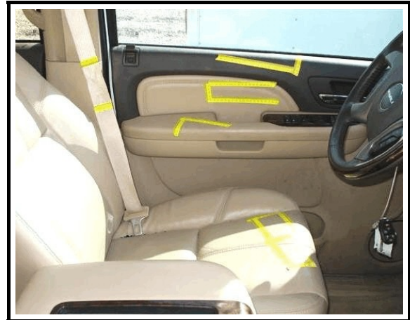
Figure 7. Areas of occupant loading and contact evidence
