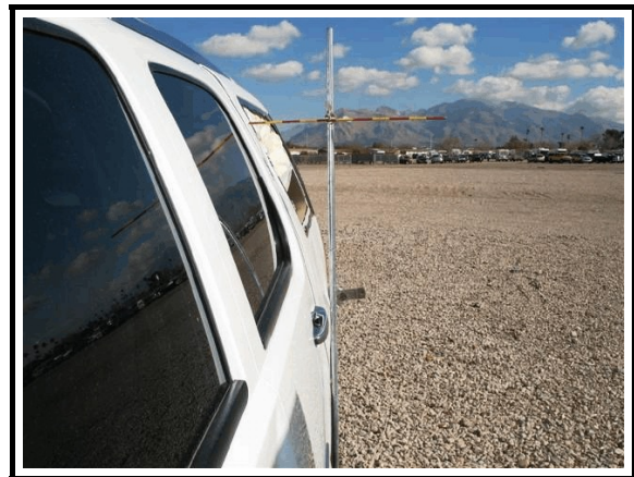
Figure 3. Maximum lateral crush measurement
