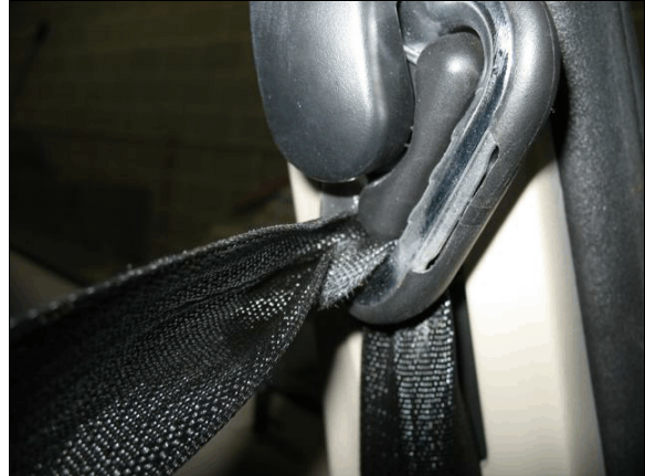
Figure 17: The driver's belt webbing entrapped in the D-ring
