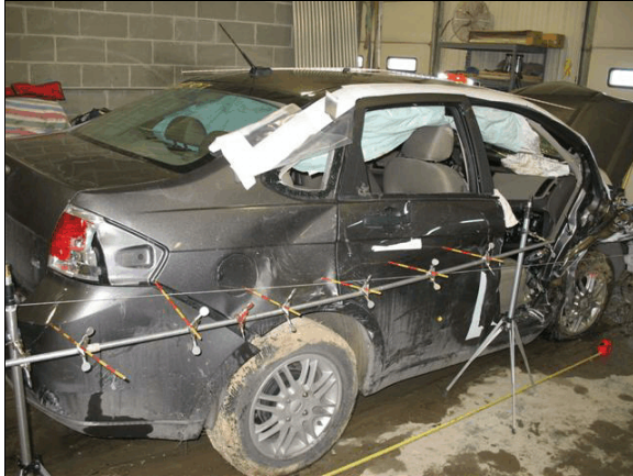
Figure 6: Damage on the right side of the Ford from impact with the left side of the Dodge
