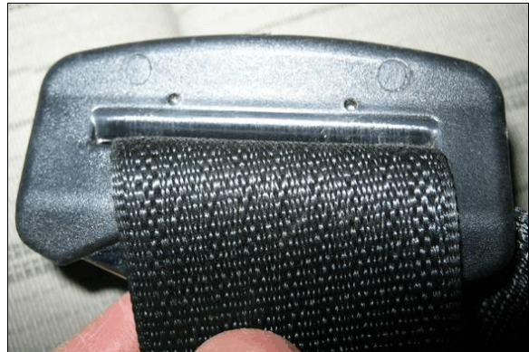
Figure 18: Load abrasions on the front passenger's latch plate belt guide
