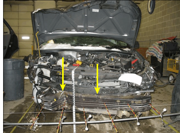
Figure 7: Arrow on right shows area of tree impact on the Ford for event 3; arrow on left shows damage from tree impact for event 5
