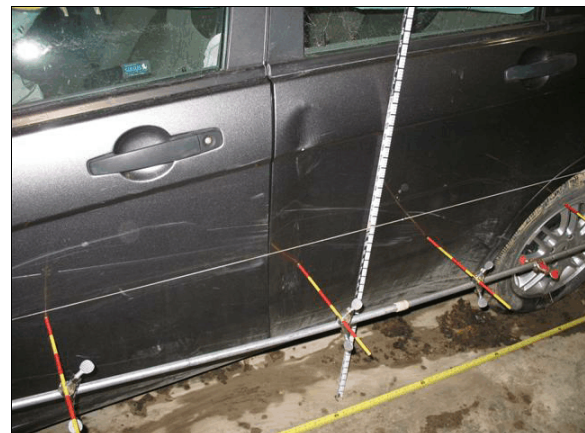
Figure 9: Sideswipe damage on the right side of the Ford from impact with a tree (event 4)
