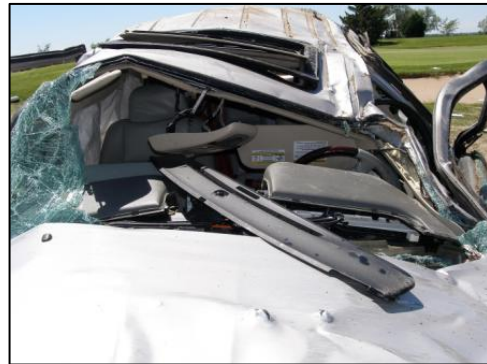
Figure 7. Vertical and lateral displacement at the left A-pillar area.
