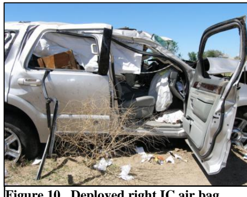
Figure 10. Deployed right IC air bag.
