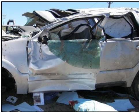
Figure 9. Deployed left IC air bag and laminated side glazing.
