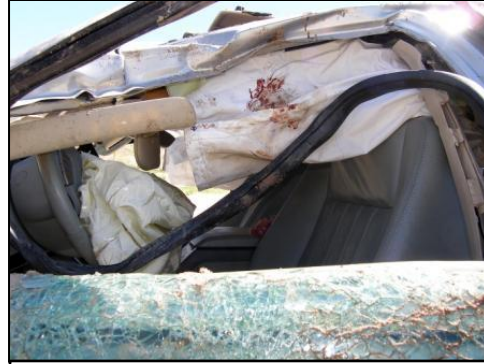
Figure 11. Driver contact evidence on the exterior of the left IC air bag and the left roof side rail.
