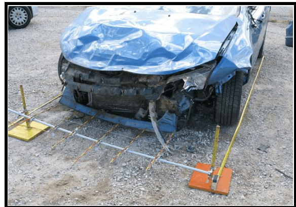
Figure 6. Front of subject vehicle with contour gauge in place, 2010 Ford Fusion
