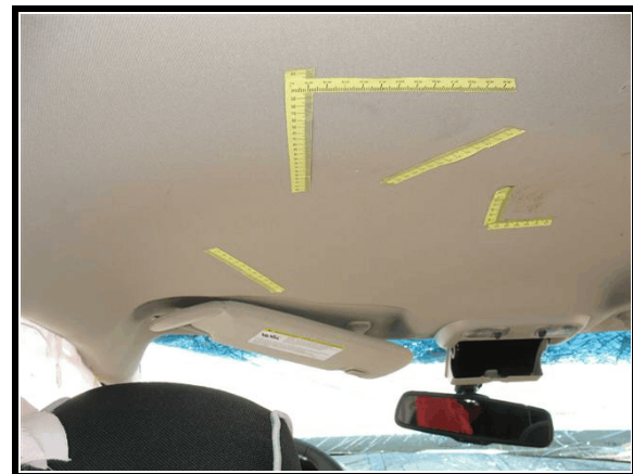
Figure 8. Possible roof contacts
