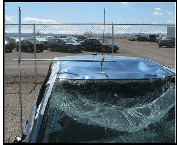
Figure 7. Maximum vertical crush, 2010 Ford Fusion
