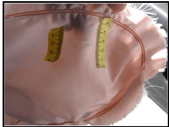
Figure 10. Contact to inboard aspect of side air bag
