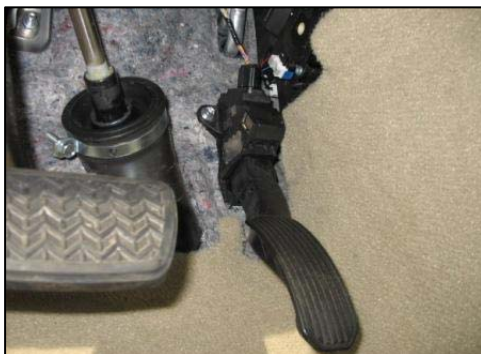
Figure 17. Overall view of the CTS accelerator pedal.
