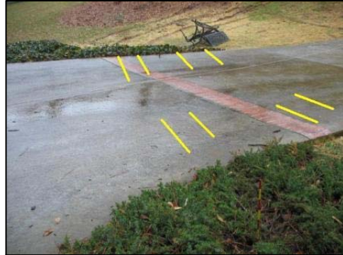
Figure 7. Acceleration tire marks across the driveway at the completion of 360 degrees of travel.
