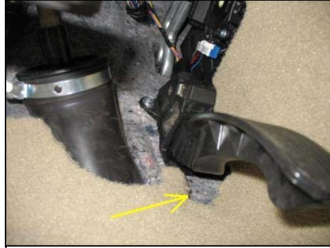
Figure 16. OEM cutout of carpet behind accelerator pedal.
