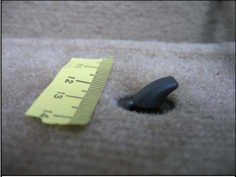
Figure 15. Hook protruding through the floor mat.
