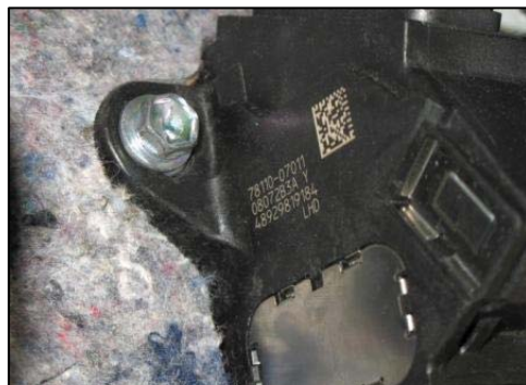
Figure 18. Identification numbers on the CTS pedal.
