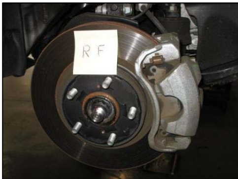
Figure 12. Right front rotor and caliper.
