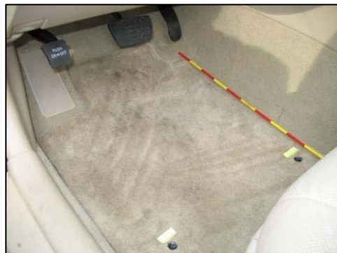
Figure 14. Position of the OEM carpeted floor mat.
