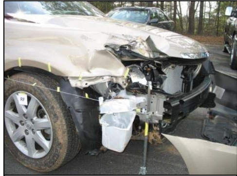
Figure 10. Tree impact damage to the right front fender area.
