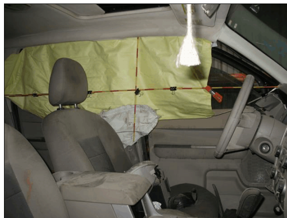
Figure 6: The Escape's left side IC air bag and seat-mounted side impact air bag
