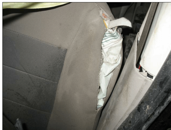
Figure 7: The Escape's left front seat back-mounted side impact deployed through a tear seam
