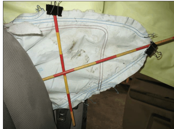
Figure 9: The deployed left front seat-mounted side impact air bag
