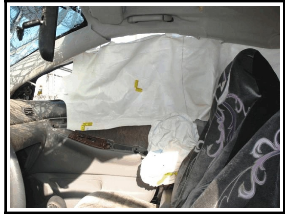
Figure 7. Right seat-mounted side air bag and right IC air bag
