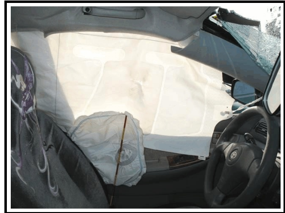
Figure 6. Left IC air bag and seat-mounted side air bag
