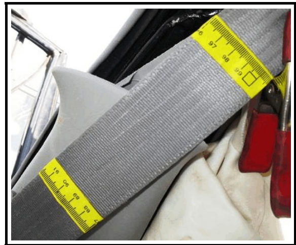
Figure 5. Front right occupant's safety belt webbing showing load marks
