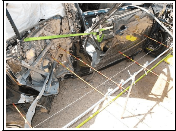
Figure 4. Right side crush profile for pole impact (Event 4)
